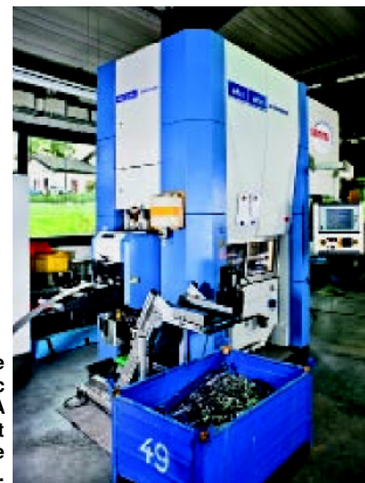
Tested and approved in three shifts: Burkhardt-automatic punching press STA with the newest Servo direct drive 'Servo III' at the Metalltechnik Annaberg Co.
