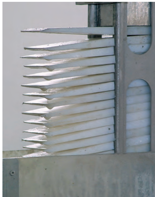
Wedge magazine with 2 x 150 wedges
