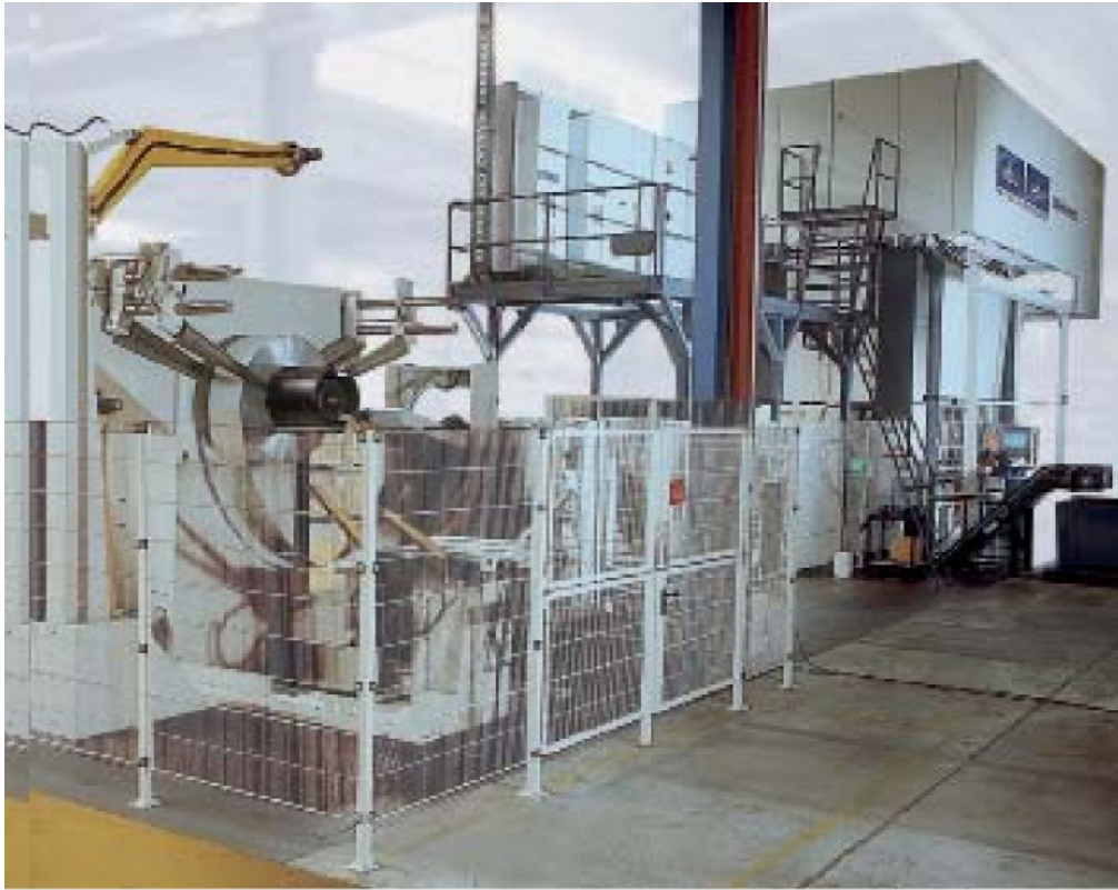
Entire Burkhardt machine system, incl. belt feeder, precision straightening machine and automatic punching press.
